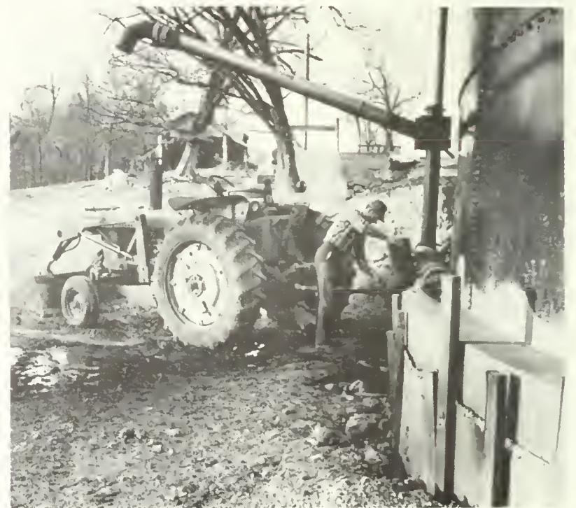
Figure 3.5.25 Tractor-operated manure pump for agitating and manure transfer from above-ground storage (courtesy A.O. Smith)
